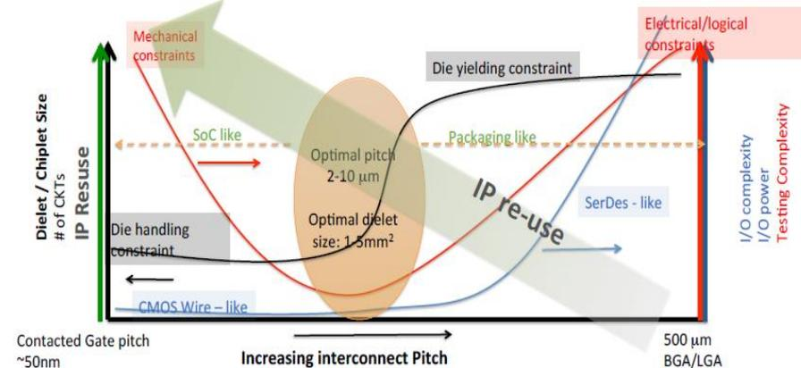
Pitch sweet spot between 2 and 10µm for chiplet (dielet) based HI platforms [3]
