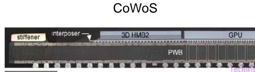
Based on inorganic RDL (silicon oxide, silicon nitride)
