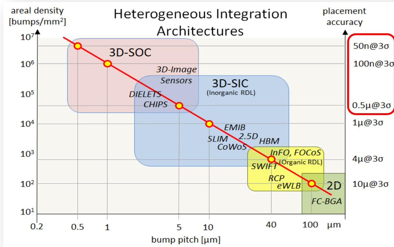
comparison of Heterogeneous Integration architectures according to bump pitch metrics and areal density
